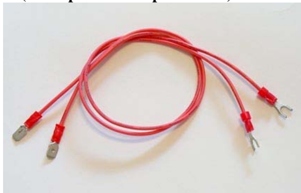
Figure 3, Cables for connecting SSR output to heater. Terminated with spade tongue terminal on one end and tab terminal on the on other end.
