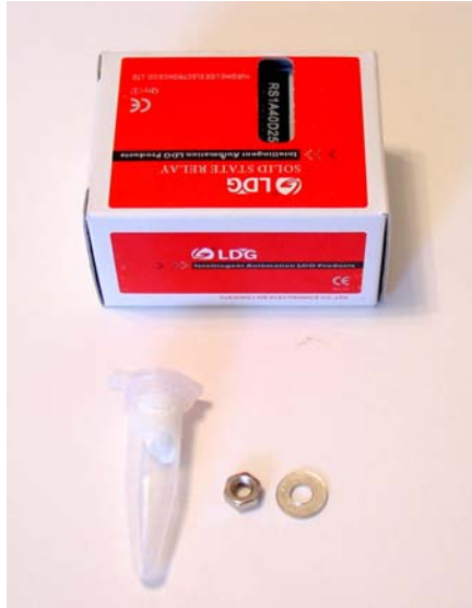
Figure 2. Solid State Relay (SSR), mounting screw nut and washer for SSR, and silicone heat transfer compound (white paste in the plastic vial) for SSR.
