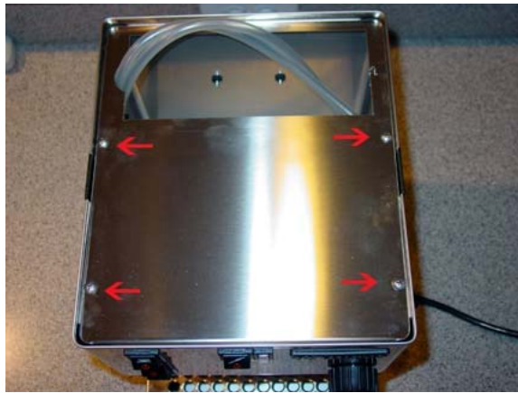
Figure 9. Top panel. Red arrows indicates the screws that hold the top panel.
