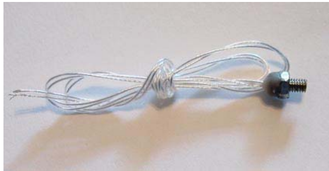
Figure 6, Temperature sensor (Pt100 RTD) with screw tip.
