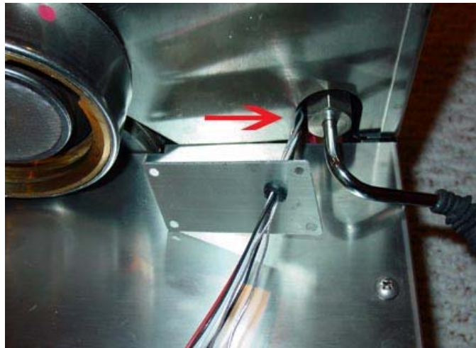
Figure 16, Cables going through the back panel of the controller box.
