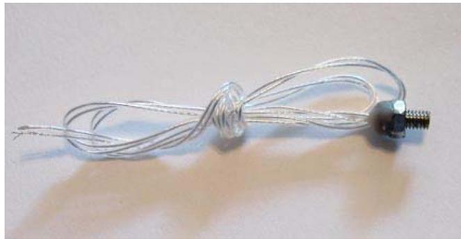
**Figure 6, Temperature sensor (Pt100 RTD) with screw tip.**
