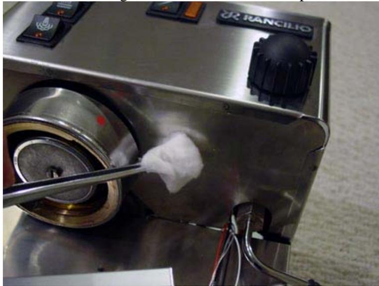
**Figure 22.** cleaning the box mounting area with alcohol.
